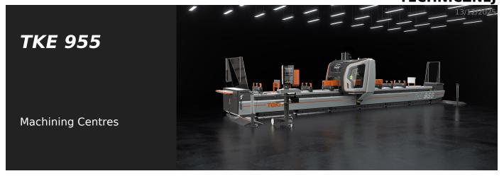
Mobile gantry 5-axis CNC machining centre for drilling, milling and tapping, at any angle from -90° to +90°, on bars or workpieces in aluminium, PVC, lightweight alloys and steel up to a thickness of 2 mm. The mobile part of the machine is composed of a dual drive gantry on a high precision rack.
