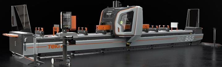
Mobile gantry 5-axis CNC machining centre for drilling, milling and tapping, at any angle from  $-90^{\circ}$  to  $+90^{\circ}$ , on bars or workpieces in aluminium, PVC, lightweight alloys and steel up to a thickness of 2 mm. The mobile part of the machine is composed of a dual drive gantry on a high precision rack.
