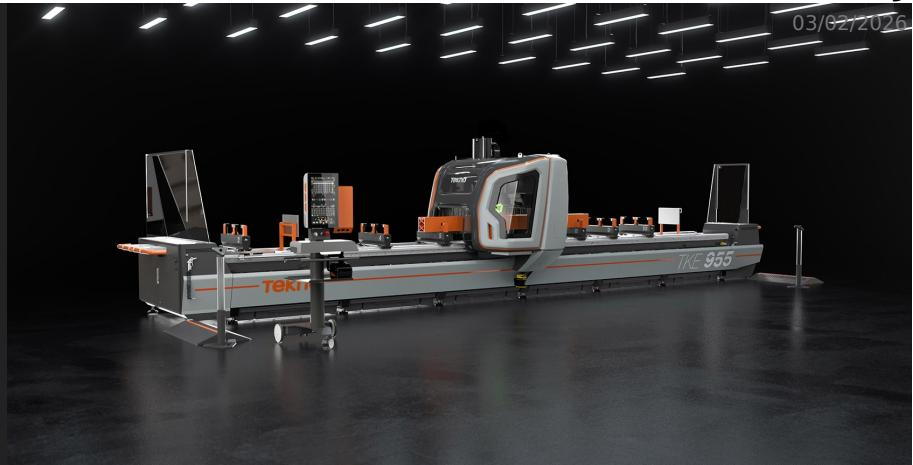
Mobile gantry 5-axis CNC machining centre for drilling, milling and tapping, at any angle from -90° to +90°, on bars or workpieces in aluminium, PVC, lightweight alloys and steel up to a thickness of 2 mm. The mobile part of the machine is composed of a dual drive gantry on a high precision rack.
