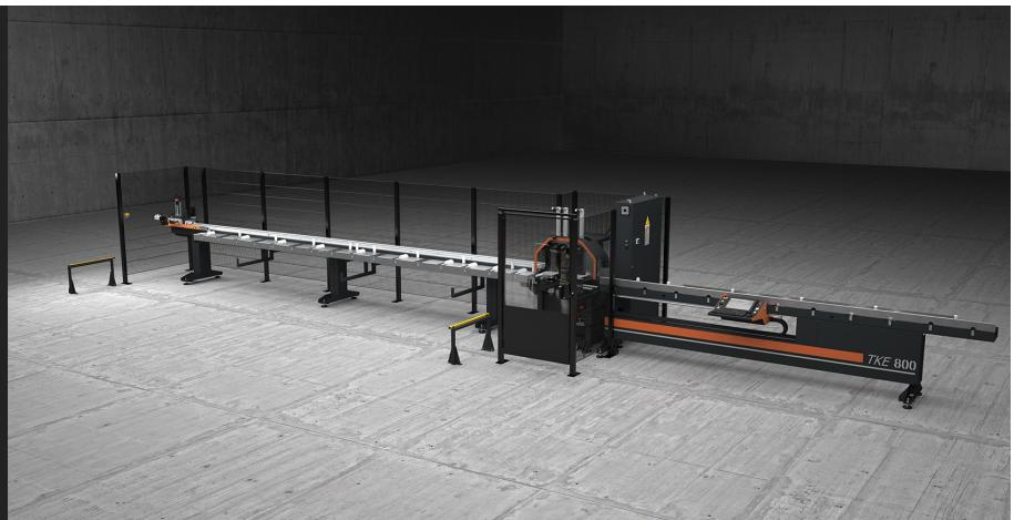
A semiautomatic version cutting centre with 2 controlled axes, manual loading/unloading on opposite sides of the machine, with front CNC blade, dedicated to cutting Aluminium and PVC profiles and light alloys in general. It performs predefined and optimised cutting lists in automatic. Designed to execute cutting at angles ranging from 45° to 135° or from 22°30' to 157°30'. Configurable with horizontal or vertical drilling units that can be personalised for specific automatic machining.
