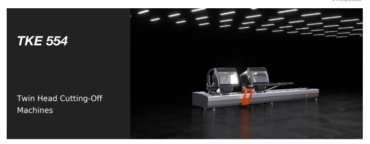
Twin-head cutting-off machine with 3 controlled axes with automatic movement of the mobile head and electronic control of every angular setting within the range 45° (internal) to 22°30' (external). The feeding of the two 550 mm blades is driven by hydro-pneumatic cylinders.
