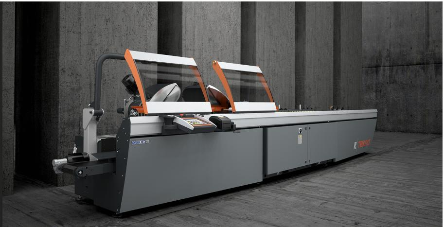
Twin-head cutting-off machine with 3 controlled axes, automatic traverse of the moving cutting head and electronic control of every angular setting from 45° (internal) to 15° (external) with accuracy of 280 places on each degree. The blade feed is controled by two hydro-pneumatic cylinders.
