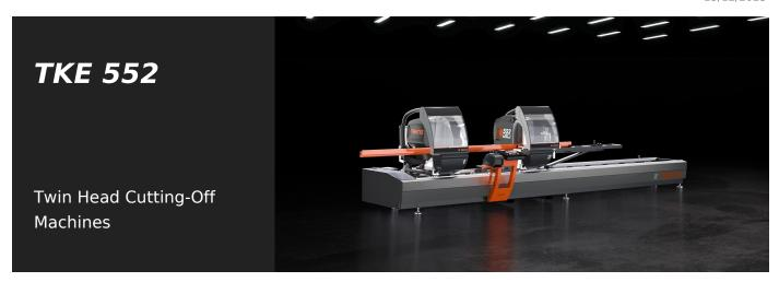
Electronic twin-head cutting-off machine with automatic traverse of the moving cutting head powered by brushless motor with numerical control system. Pneumatic tilting of cutting units from 90° to 22°30′ (outward) in two fixed positions or with optional mechanical adjustment system for intermediate angles. Hydro-pneumatic blade feed.
