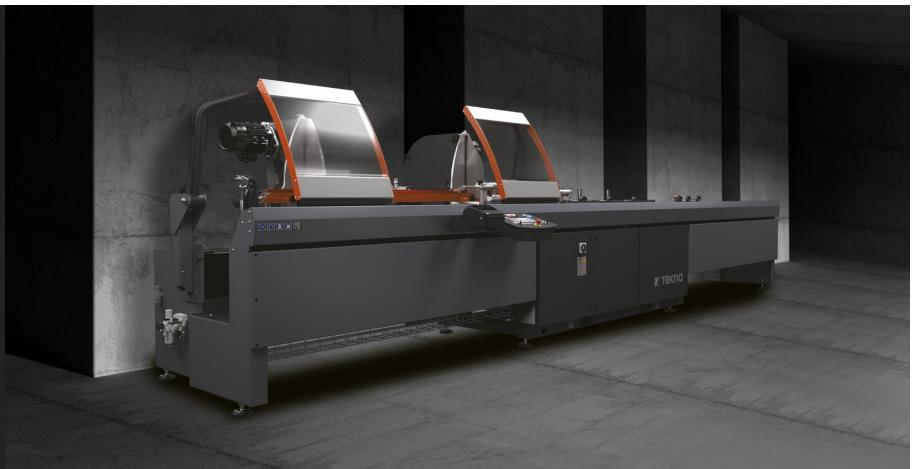
Electronic twin-head cutting-off machine with automatic traverse of the moving cutting head powered by brushless motor with numerical control system. Pneumatic control of the angular setting from 90° to 22°30' (external) with mechanic adjustment of intermediate angles. Hydro-pneumatic blade feed.
