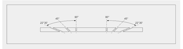
Mechanical adjustment of intermediate angles
