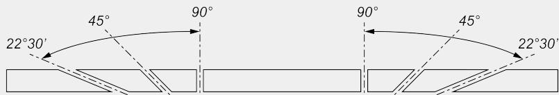
Mechanical adjustment of intermediate angles
