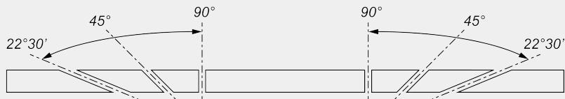
Mechanical adjustment of intermediate angles
