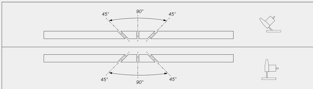
Mechanical adjustment of intermediate angles
