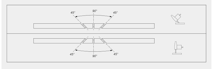
Mechanical adjustment of intermediate angles
