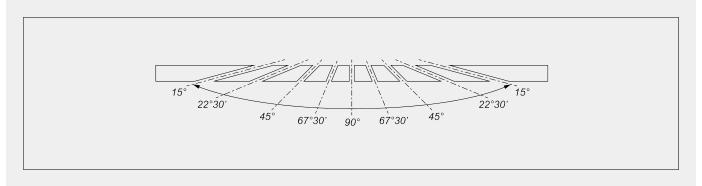
Mechanical adjustment of intermediate angles
