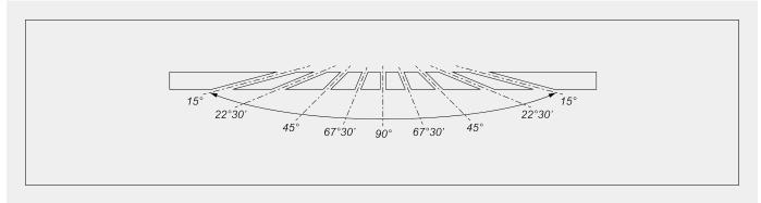
Mechanical adjustment of intermediate angles
