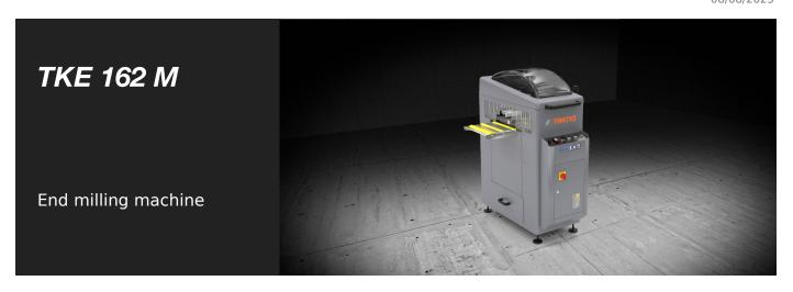
TKE 162 M is a horizontal end milling machine with manual feed. Milling of intermediate angles,  $+45^{\circ}$  /  $90^{\circ}$  /  $-45^{\circ}$ . High tool speed, 6000 rpm, for improved standard of machining on the painted profile and with intermediate angles. Quick tool change with pneumatic control. Scratch-proof table. Full guarding of work zone with ample internal visibility.
