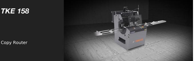
Manually controlled single head copy router with pneumatic clamping and traverse of the head with indirect lever. Tool rotation speed editable with electronic inverter to allow the machining of steel up to 2 mm, and to improve the quality of milling and tool life. Ability to run through machining of aluminum without turning the workpiece. Scratch-proof. Manually controlled stylus.
