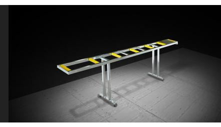
Structure in steel tubular con adjustable feet and PVC-coated steel rollers. 3.500 mm-long roller conveyors with 240 mm rollers, or 4.000 mm-long with 440 mm rollers. Unloading roller conveyors equipped with metric rod and measuring lock.
