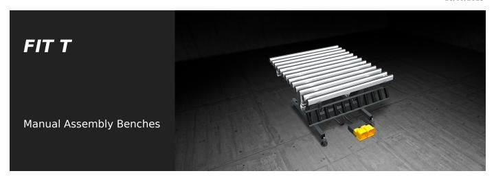
Sash and casement assembly bench. Tilting table from 0° (horizontal) to 85°, with pneumatic exchange between the soft PVC resting surface (for assembly operations) and the anti-friction hard PVC resting surface (for handling operations). The roller conveyor can be manually tilted and it is adjustable in height (from 170 to 460 mm) independently from the work table height. The work table height is adjustable from 895 to 965 mm and the mounting feet are complete with holes for floor anchoring.
