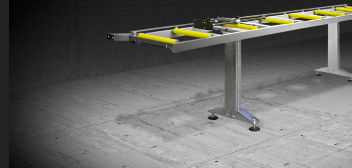
Tubular steel construction with adjustable mounting feet and PVC covered steel rolls. In the version with rolls size 240 mm, roller conveyor length is 3.500 mm; with rolls size 440 mm, roller conveyor length is 4.000 mm.
