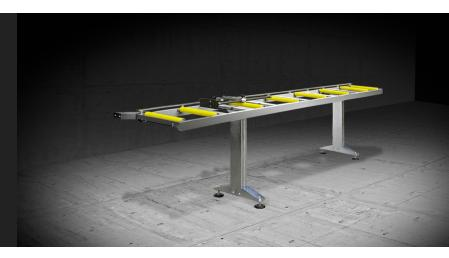
Tubular steel construction with adjustable mounting feet and PVC covered steel rolls. In the version with rolls size 240 mm, roller conveyor length is 3.500 mm; with rolls size 440 mm, roller conveyor length is 4.000 mm.
