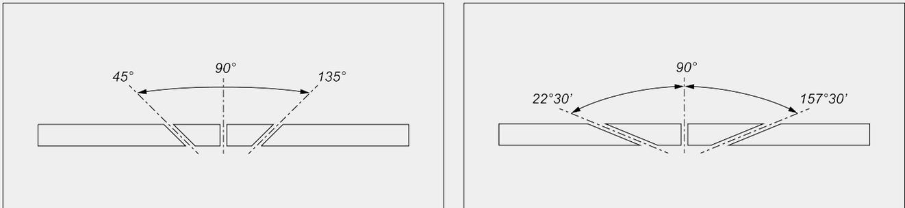
Electronic adjustment of intermediate angles
