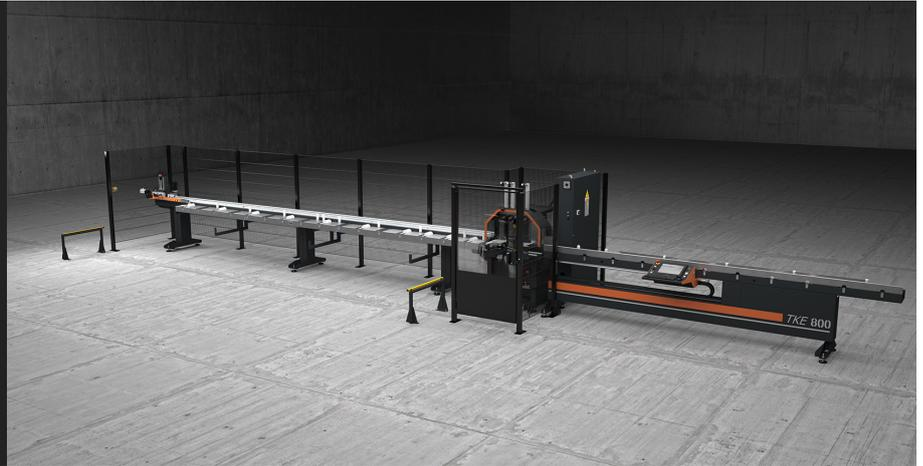
A semiautomatic version cutting centre with 2 controlled axes, manual loading/unloading on opposite sides of the machine, with front CNC blade, dedicated to cutting Aluminium and PVC profiles and light alloys in general. It performs predefined and optimised cutting lists in automatic. Designed to execute cutting at angles ranging from 45° to 135° or from 22°30' to 157°30'. Configurable with horizontal or vertical drilling units that can be personalised for specific automatic machining.
