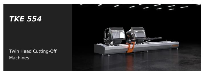
Twin-head cutting-off machine with 3 controlled axes with automatic movement of the mobile head and electronic control of every angular setting within the range 45° (internal) to 22°30' (external). The feeding of the two 550 mm blades is driven by hydro-pneumatic cylinders.
