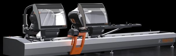
Twin-head cutting-off machine with 3 controlled axes with automatic movement of the mobile head and electronic control of every angular setting within the range 45° (internal) to 22°30' (external). The feeding of the two 550 mm blades is driven by hydro-pneumatic cylinders.
