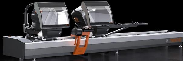
Twin-head cutting-off machine with 3 controlled axes with automatic movement of the mobile head and electronic control of every angular setting within the range 45° (internal) to 22°30' (external). The feeding of the two 550 mm blades is driven by hydro-pneumatic cylinders.
