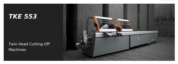
Twin-head cutting-off machine with 3 controlled axes, automatic traverse of the moving cutting head and electronic control of every angular setting from 45° (internal) to 15° (external) with accuracy of 280 places on each degree. The blade feed is controlled by two hydro-pneumatic cylinders.
