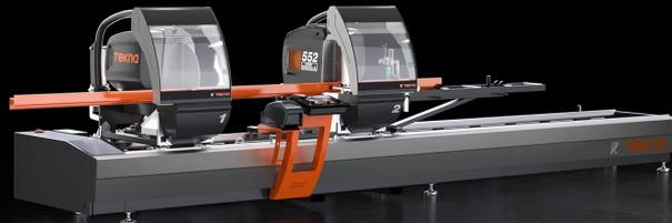
Electronic twin-head cutting-off machine with automatic traverse of the moving cutting head powered by brushless motor with numerical control system. Pneumatic tilting of cutting units from 90° to 22°30' (outward) in two fixed positions or with optional mechanical adjustment system for intermediate angles. Hydro-pneumatic blade feed.
