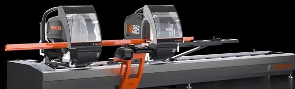
Electronic twin-head cutting-off machine with automatic traverse of the moving cutting head powered by brushless motor with numerical control system. Pneumatic tilting of cutting units from 90° to 22°30' (outward) in two fixed positions or with optional mechanical adjustment system for intermediate angles. Hydro-pneumatic blade feed.
