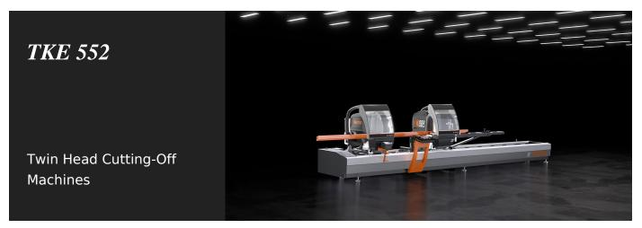
Electronic twin-head cutting-off machine with automatic traverse of the moving cutting head powered by brushless motor with numerical control system. Pneumatic tilting of cutting units from 90° to 22°30' (outward) in two fixed positions or with optional mechanical adjustment system for intermediate angles. Hydro-pneumatic blade feed.
