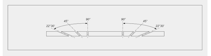
Mechanical adjustment of intermediate angles
