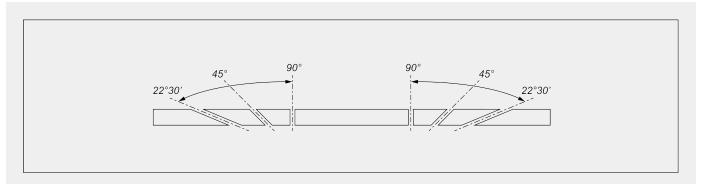
Mechanical adjustment of intermediate angles
