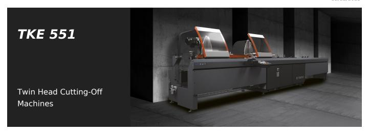
Electronic twin-head cutting-off machine with automatic traverse of the moving cutting head powered by brushless motor with numerical control system. Pneumatic control of the angular setting from 90° to 22°30′ (external) with mechanic adjustment of intermediate angles. Hydro-pneumatic blade feed.
