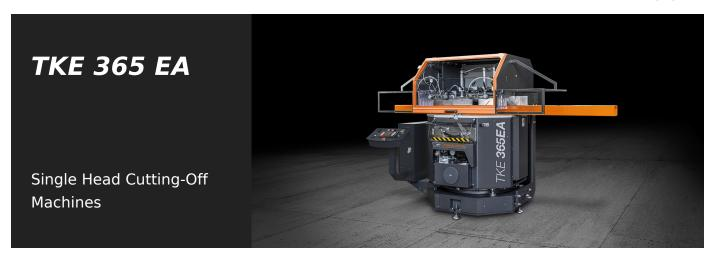
Single-head, rising blade cutting-off machine, with N/C automatic rotation of the vertical axis through brushless motor and contemporaneous hydraulic tilting of the horizontal axis. Cutting with angular settings from 90° to 22°30′ (left and right) on the vertical axis and from 90° to 35° (right only) on the horizontal axis.
