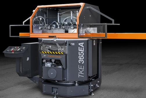
Single-head, rising blade cutting-off machine, with N/C automatic rotation of the vertical axis through brushless motor and contemporaneous hydraulic tilting of the horizontal axis. Cutting with angular settings from 90° to 22°30' (left and right) on the vertical axis and from 90° to 35° (right only) on the horizontal axis.
