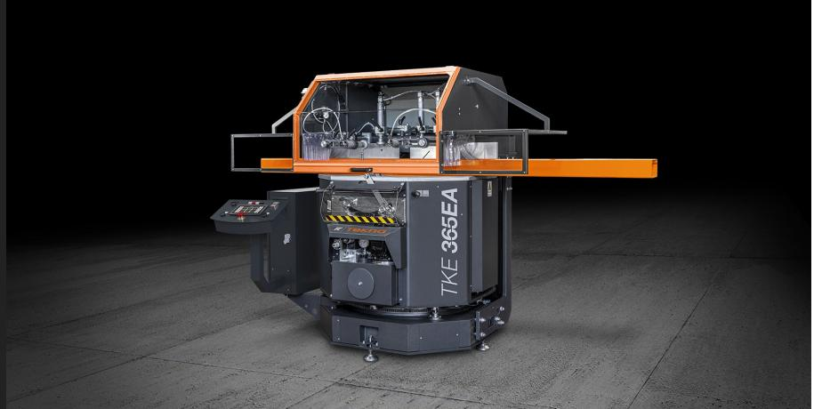
Single-head, rising blade cutting-off machine, with N/C automatic rotation of the vertical axis through brushless motor and contemporaneous hydraulic tilting of the horizontal axis. Cutting with angular settings from 90° to 22°30' (left and right) on the vertical axis and from 90° to 35° (right only) on the horizontal axis.
