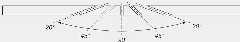
Mechanical adjustment of intermediate angles
