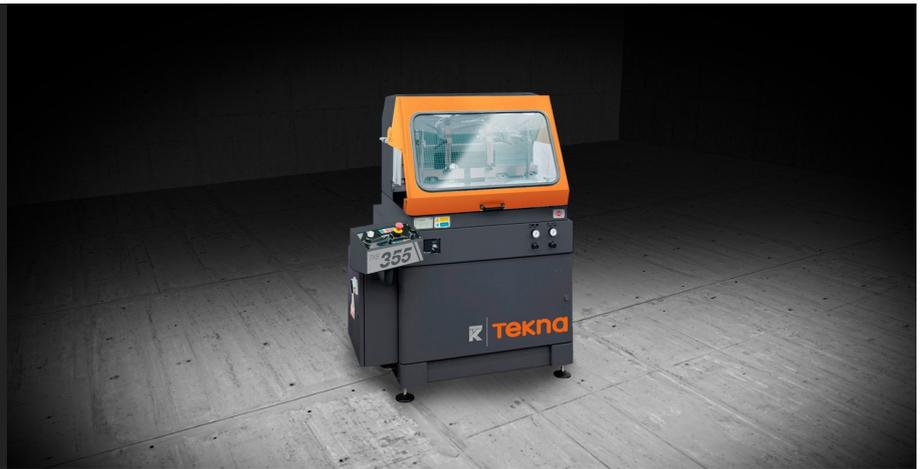
Single head, rising blade cutting-off machine, with left loading side, for cutting at angular settings from 20° to the left to 20° to the right as intermediate angles.
