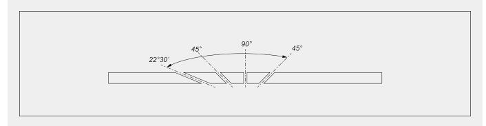
Mechanical adjustment of intermediate angles
