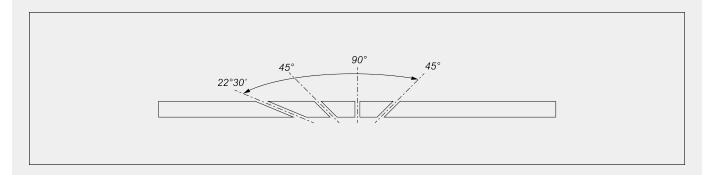
Mechanical adjustment of intermediate angles
