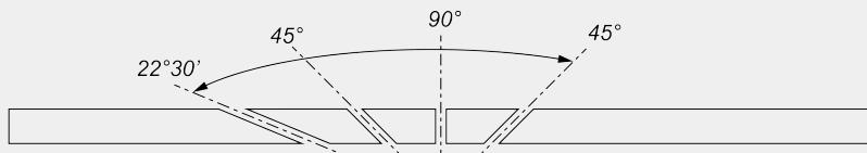
Mechanical adjustment of intermediate angles
