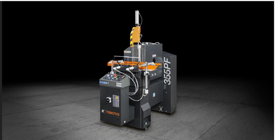
Single head cutting-off machine with horizontal blade feed and left loading side, pneumatic double side tilting of the cutting head in fixed positions: 45° to the left plus 90°, 45° and 22°30' to the right. A special positive stop also allows cutting at intermediate angles.
