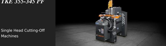
Single head cutting-off machine with horizontal blade feed and left loading side, pneumatic double side tilting of the cutting head in fixed positions: 45° to the left plus 90°, 45° and 22°30' to the right. A special positive stop also allows cutting atintermediate angles.
