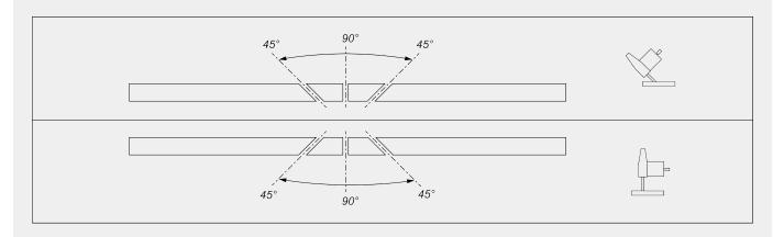
Mechanical adjustment of intermediate angles
