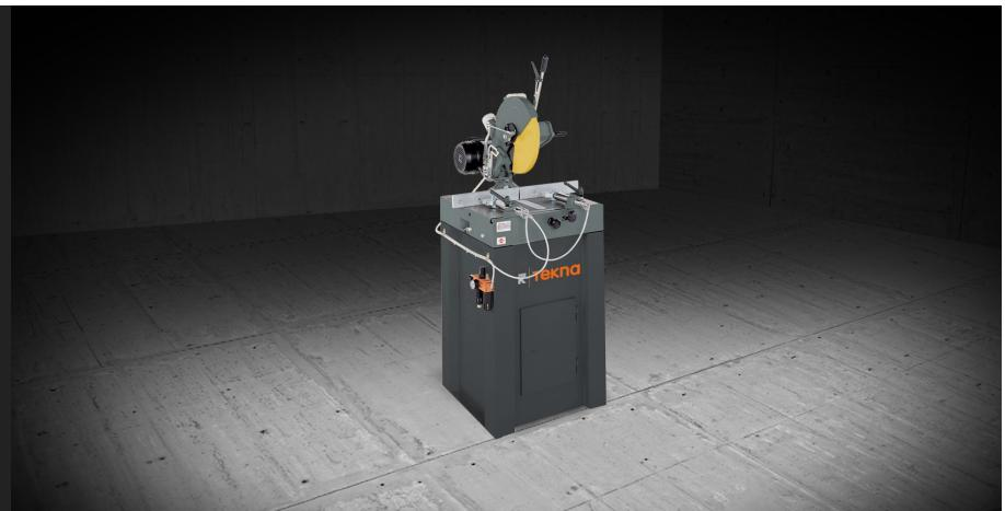
Single head chop saw (downstroking cutting-off machine) with left loading side, rotation of the cutting head by 45° (to right and left) and manual tilting by 45° about the horizontal axis.
