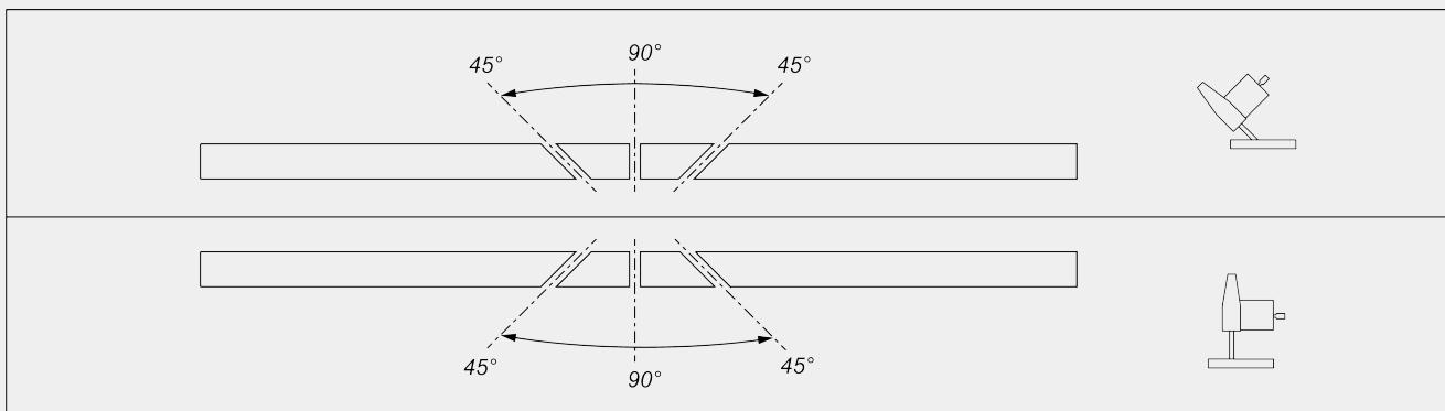
Mechanical adjustment of intermediate angles
