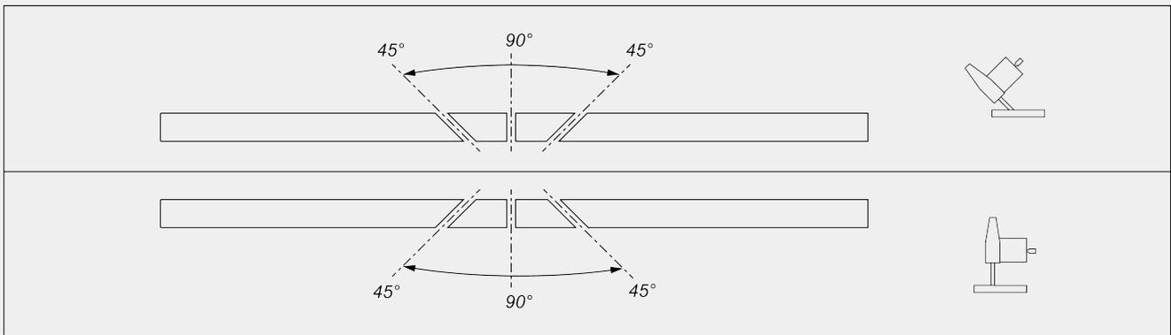
Mechanical adjustment of intermediate angles
