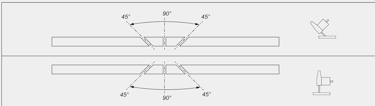
Mechanical adjustment of intermediate angles
