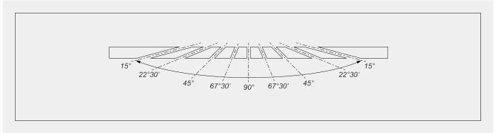
Mechanical adjustment of intermediate angles
