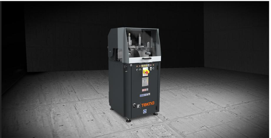
Single-head cutting-off machine with rising blade and pneumatic feed, with left loading side, able to perform cuts from 15° left to 15° right and intermediate angles.
