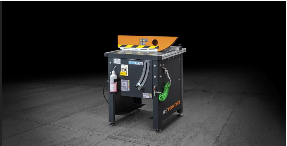
Single head rising blade trimming machine, for extruded profiles and flat sheets made of aluminium. The especially rugged structure allows very sharp and accurate cutting in order to obtain exactly parallel faces of the profiles. Furthermore the machine can be set-up with support roller conveyors to extend its versatility. The blade guard has been designed and developed to ensure working under the best possible conditions of safety.
