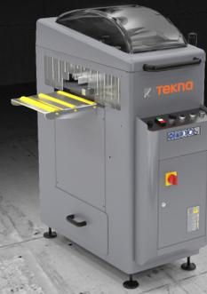
TKE 162 M is a horizontal end milling machine with manual feed. Milling of intermediate angles,  $+45^\circ / 90^\circ / -45^\circ$ . High tool speed, 6000 rpm, for improved standard of machining on the painted profile and with intermediate angles. Quick tool change with pneumatic control. Scratch-proof table. Full guarding of work zone with ample internal visibility.
