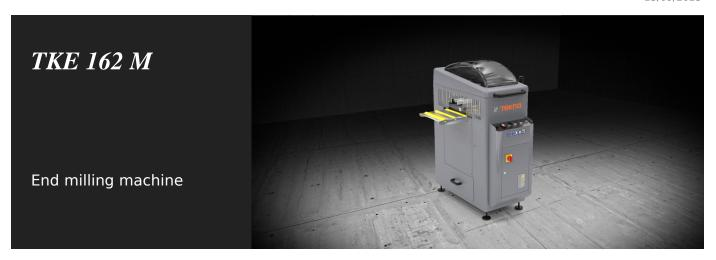
TKE 162 M is a horizontal end milling machine with manual feed. Milling of intermediate angles, +45° / 90° / -45°. High tool speed, 6000 rpm, for improved standard of machining on the painted profile and with intermediate angles. Quick tool change with pneumatic control. Scratch-proof table. Full guarding of work zone with ample internal visibility.
