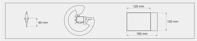
Maximum machinable section on 4 sides – L x H (mm) 120 x 100
