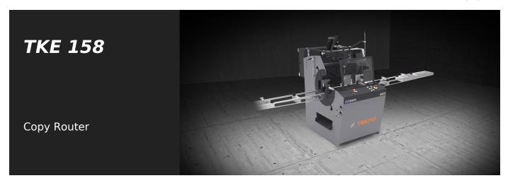
Manually controlled single head copy router with pneumatic clamping and traverse of the head with indirect lever. Tool rotation speed editable with electronic inverter to allow the machining of steel up to 2 mm, and to improve the quality of milling and tool life. Ability to run through machining of aluminum without turning the workpiece. Scratch-proof. Manually controlled stylus.
