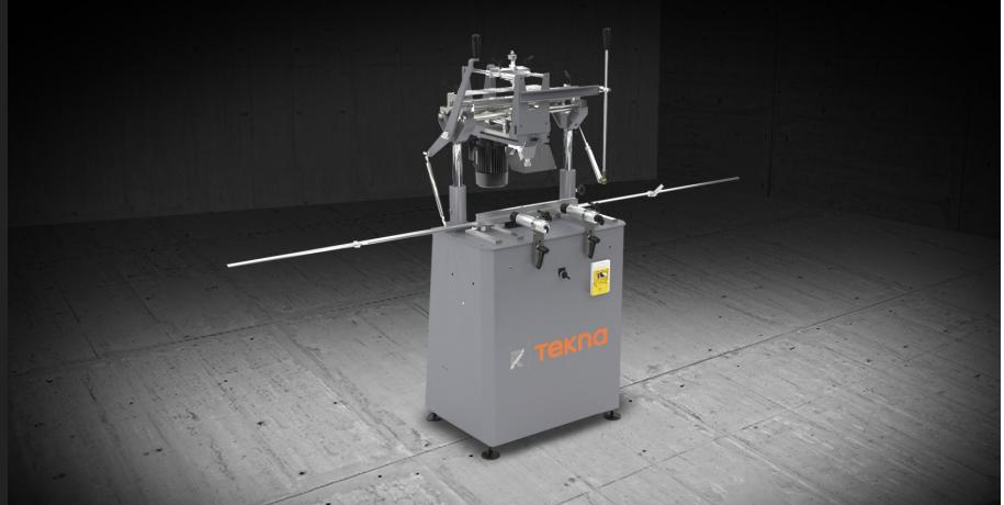
Single-head copy router with manual downfeed. Manually controlled single-head copy router with pneumatic clamping and traverse of the cutting head with indirect lever. Predisposition for performing through machining operations on aluminium without turning the workpiece and for working steel up to 2 mm. Scratch-proof work table. Pneumatic stylus with control on the handle.
