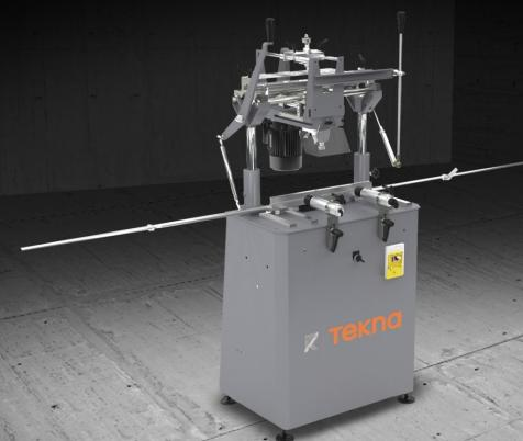
Single-head copy router with manual downfeed. Manually controlled single-head copy router with pneumatic clamping and traverse of the cutting head with indirect lever. Predisposition for performing through machining operations on aluminium without turning the workpiece and for working steel up to 2 mm. Scratch-proof work table. Pneumatic stylus with control on the handle.
