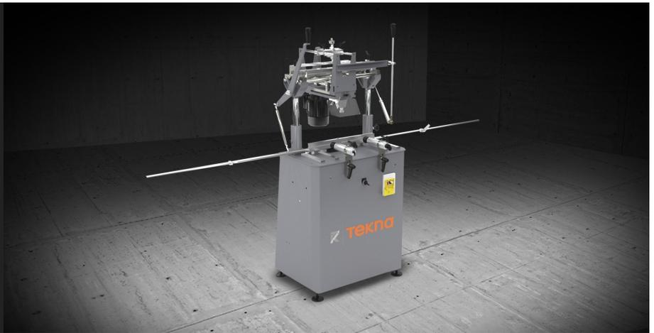
Single-head copy router with manual downfeed. Manually controlled single-head copy router with pneumatic clamping and traverse of the cutting head with indirect lever. Predisposition for performing through machining operations on aluminium without turning the workpiece and for working steel up to 2 mm. Scratch-proof work table. Pneumatic stylus with control on the handle.
