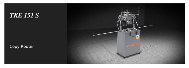
Single-head copy router with manual downfeed. Manually controlled single-head copy router with pneumatic clamping and traverse of the cutting head with indirect lever. Predisposition for performing through machining operations on aluminium without turning the workpiece and for working steel up to 2 mm. Scratch-proof work table. Pneumatic stylus with control on the handle.
