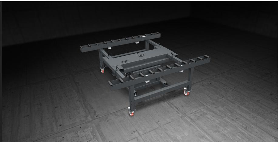
Modular bench for assembly and in-line handling of curtain wall frames. It is provided with two roller tracks covered with soft PVC sheathing; the distance between the two tracks is adjustable according to the width of the curtain wall section. A pneumatically operated system allows clamping the rollers during the work phases. The entire bench can be rotated by 360° in order to facilitate the assembly and sealing of the curtain wall; the angular position is clamped pneumatically.
