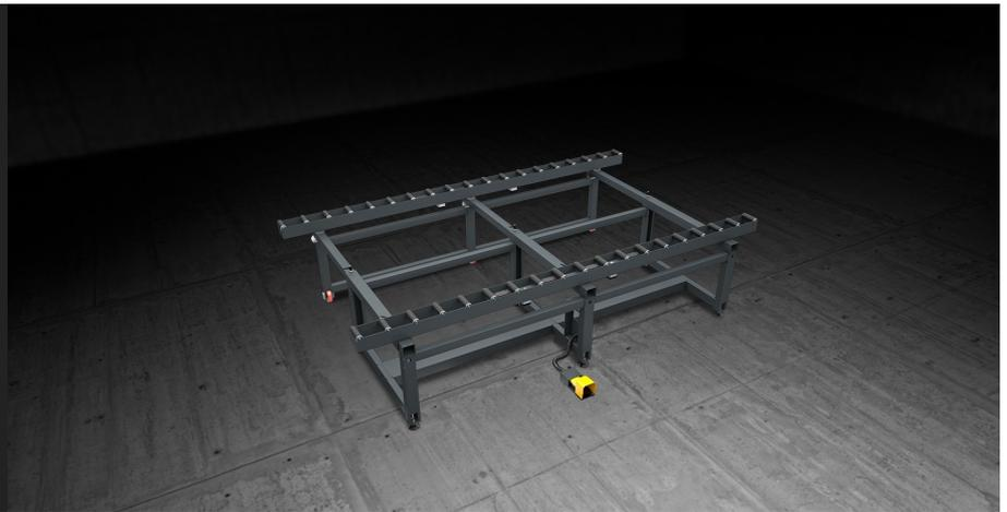
Large size modular bench for assembly and in-line handling of curtain wall frames. It is provided with two roller tracks covered with soft PVC sheathing; the distance between the two tracks is adjustable according to the width of the curtain wall section. A pneumatically operated system allows clamping the rollers during the work phases.
