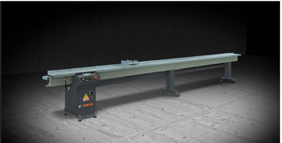
Stop gauge and profile support system, driven by DC motor, complete with electronic read-out through encoder.
