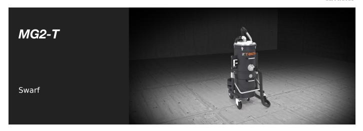
Extraction system for aluminium and PVC swarf with single suction nozzle, designed for cleaning machines and the work environment or extract swarf from work units that require high vacuum values. The use of a high-depression side duct turbine makes it suitable for various extraction requirements. Equipped with an anti-static filter, this is a wheel-mounted, quick-release, automatic vibrating filter and collection tank cleaning system, to dispose of exhausted material easily and quickly.
