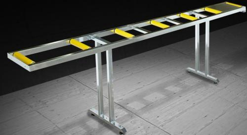
Structure in steel tubular con adjustable feet and PVC-coated steel rollers. 3.500 mm-long roller conveyors with 240 mm rollers, or 4.000 mm-long with 440 mm rollers. Unloading roller conveyors equipped with metric rod and measuring lock.
