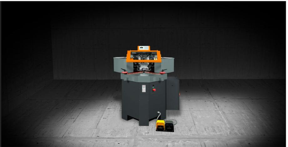
The machine has two special operating heads equipped with masses in which the 2 knives are adjustable on all crimping positions. The knives move and are adjustable on the Y axis (along the profile), on the Z axis (top-bottom) and on the X axis (along the crimping direction). These conditions prevent the replacement of tools on the machine regardless of the different types of profiles. In this way, the times and costs of placing are reduced.
