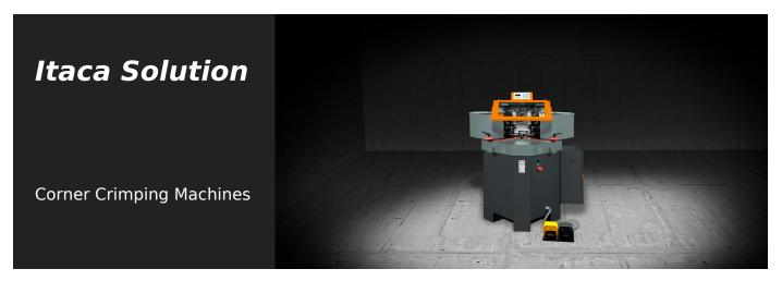
The machine has two special operating heads equipped with masses in which the 2 knives are adjustable on all crimping positions. The knives move and are adjustable on the Y axis (along the profile), on the Z axis (top-bottom) and on the X axis (along the crimping direction). These conditions prevent the replacement of tools on the machine regardless of the different types of profiles. In this way, the times and costs of placing are reduced.
