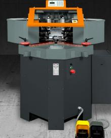
The machine has two special operating heads equipped with masses in which the 2 knives are adjustable on all crimping positions. The knives move and are adjustable on the Y axis (along the profile), on the Z axis (top-bottom) and on the X axis (along the crimping direction). These conditions prevent the replacement of tools on the machine regardless of the different types of profiles. In this way, the times and costs of placing are reduced.
