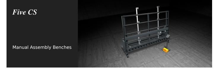
Test bench for frames in aluminium. It allows re-create the conditions of use of the frame. The casement is locked by a system of vices adjustable throughout the casement height; the operator can assemble the sash and the glass inside the casement and finally test it. The roller conveyor allows the operator to feed/outfeed heavy frames in complete autonomy.
