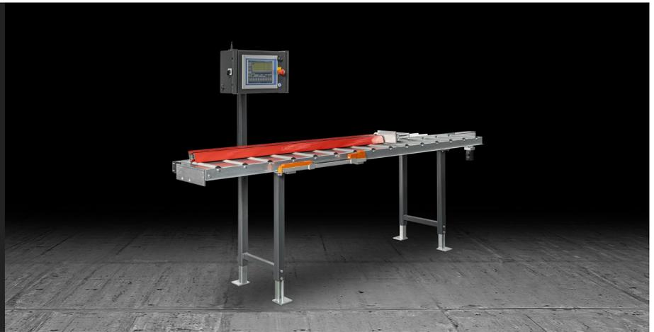
Stop gauge and profile support system with movement of the stop on CN axis and electronic read-out by absolute magnetic band. Equipped with an electronic measurement system that allows to save data on internal memory or transferred in real time to a PC or to the control unit of a miter saw via Bluetooth. It allows machining with high accuracy and repeatability of positioning.
