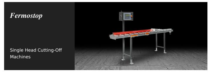
Stop gauge and profile support system with movement of the stop on CN axis and electronic read-out by absolute magnetic band. Equipped with an electronic measurement system that allows to save data on internal memory or transferred in real time to a PC or to the control unit of a miter saw via Bluetooth. It allows machining with high accuracy and repeatability of positioning.
