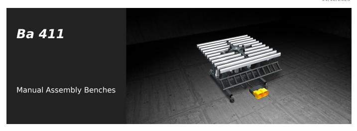
Assembly bench for glazed sashes with work table tilting from 0° (horizontal) to 85°. The drop-away roller conveyor is adjustable in height (from 170 to 460 mm) independently from the work table. The work table is adjustable from 895 to 965 mm while the feet are drilled with holes for fl oor anchoring. The bench is provided with a central spider clamp for hoisting and positioning the glass.
