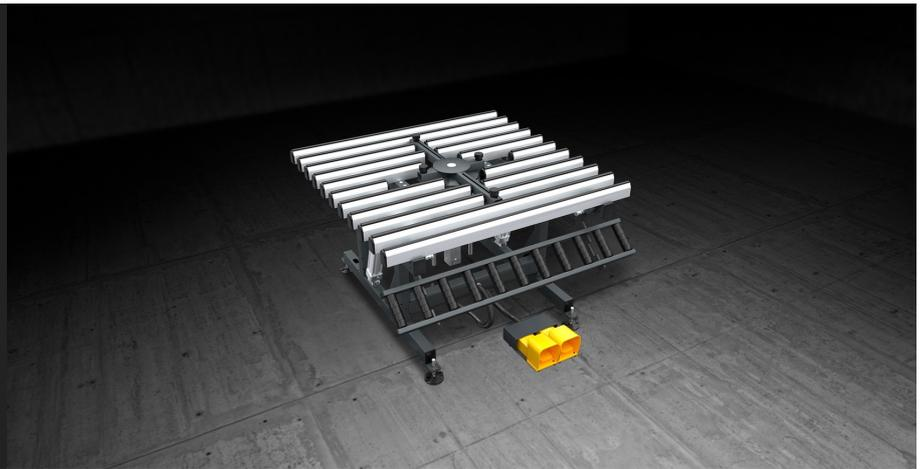
Assembly bench for glazed sashes with work table tilting from 0° (horizontal) to 85°. The drop-away roller conveyor is adjustable in height (from 170 to 460 mm) independently from the work table. The work table is adjustable from 895 to 965 mm while the feet are drilled with holes for floor anchoring. The bench is provided with a central spider clamp for hoisting and positioning the glass.
