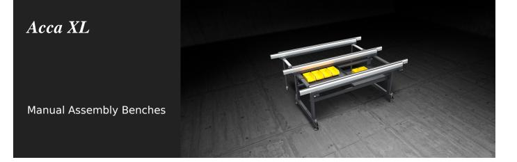
The bench is suitable for any fitting and assembly operation of door and window frames. The sliding and extendable tops allow operations with every size frames and very big structures in complete safety.
